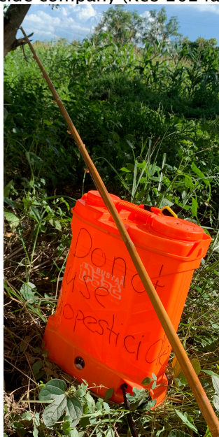
Figure 12: The electric knapsack sprayer BUSTAR BS-20D 20 L with the spraying bar which was used in the on station trial as well as in the on farm trial
